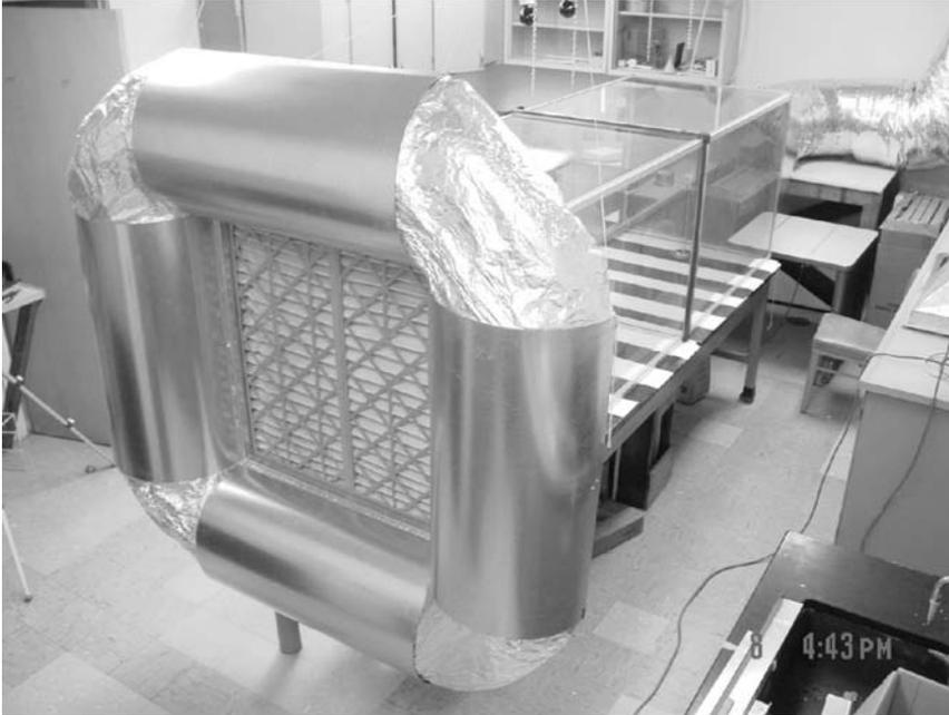
Fig. 27. Wind tunnel for assessing flight behavior of codling moth.
