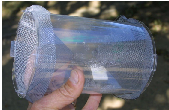
Figure 2. Improved version of the experimental Trece double cone trap, with a plastic ring fitted to top and bottom to secure the cone screen on top and bottom instead of a rubber band and staples. This trap has adhesive on the inside to keep BMSB in the trap.
