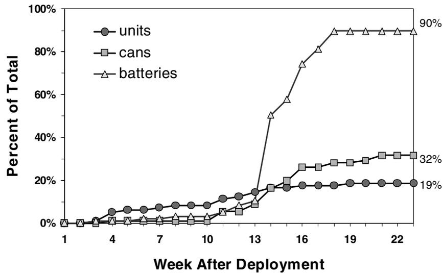
Figure 4. Cumulative replacement rate for components of the Paramount Puffer over time.
