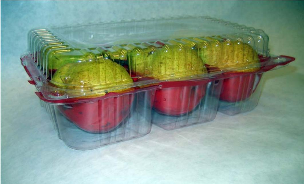
Figure 2. Photo of suspended tray clamshell package (Hammock pack) used in test
