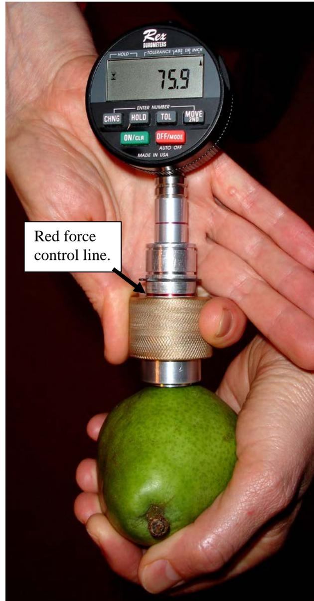
Figure 3. Force control mechanism mounted on an 'E' durometer. The operator slides the outer ring toward the fruit until the red force control line appears.
